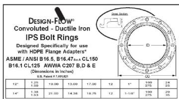
WPR (working pressure rating) is for free-floating rings on HDPE flange adapters and includes a 2:1 safety factor. These are cast convoluted ductile iron metal bolt rings with 150# bolt-hole pattern; the material is in compliance with ASTM A536 GR 65/45/12 and surfaced in Bright Red oil based enamel paint.
